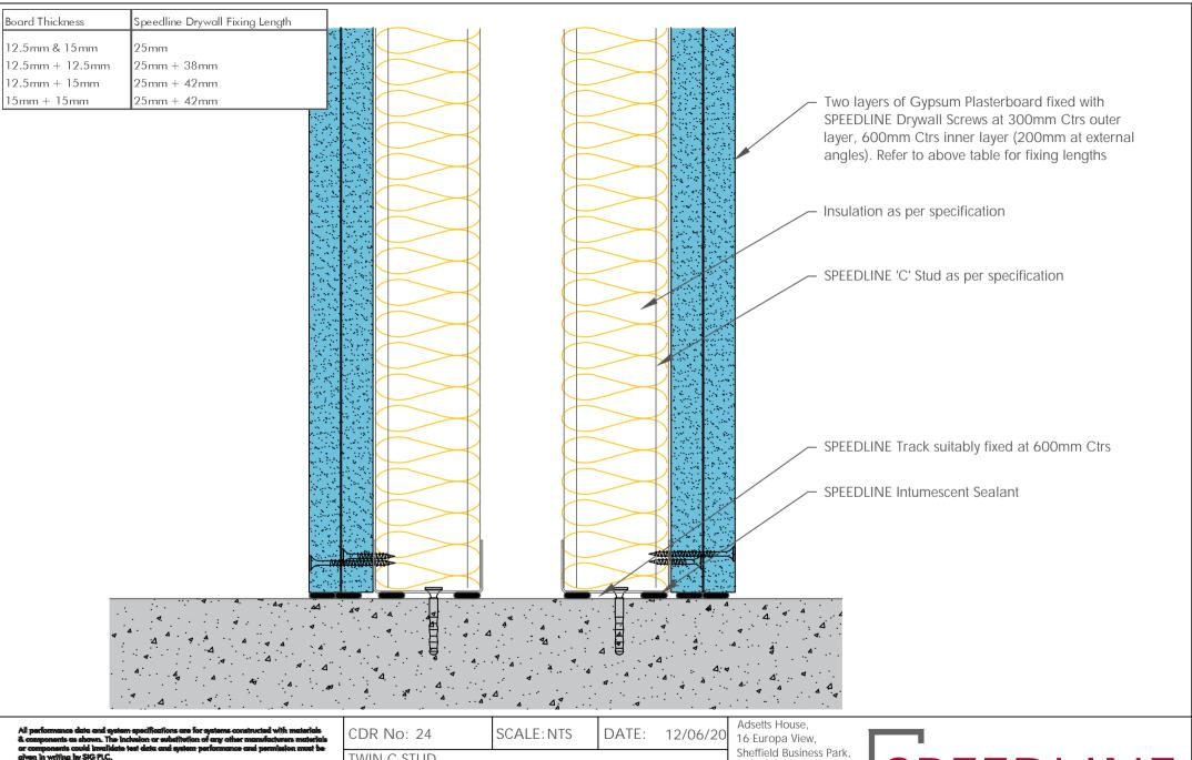
TWIN C STUD BASE DETAIL **DOUBLE LAYER** 502x15SRIns Details to be read in conjunction with project specification guidelines
